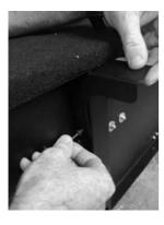
Place the Draw System into the vehicle lining up the front of the Draw System with the edge of the load bay area. There should be a slight gap between the Draw System and the interior door flap when the flap is in the upright position.
