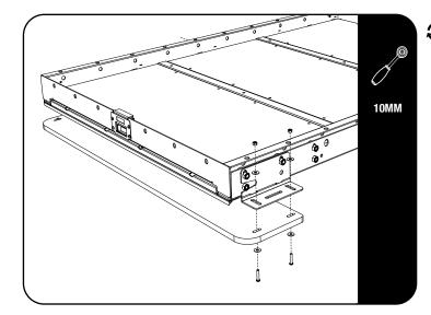
Before fitting the Cargo Slide in the vehicle, remove the protective wood base by loosening the four M6 button heads.
