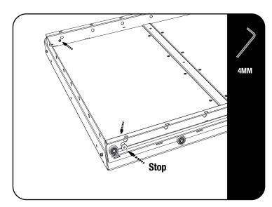
Looking at both the left and right rear corners of the Cargo Slide (Item 1), loosen and remove the rubber stopper. this is done by gripping the stopper to prevent it from turning and removing the M6 button head bolt as shown. Once removed keep in a safe place as you will need to replace them at a later stage.
