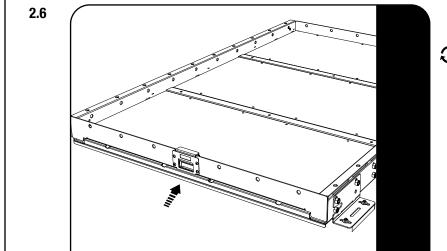
Refer to Step 2.2, refit the tray and stoppers. Once refitted check that the push to close latch engages fully and that the slide is secure.
