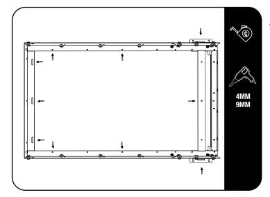
Make sure you have closed the load bed door to ensure that it does not make contact with the frame. Once you are satisfied with the positioning of the frame, mark the position of all the mounting points as indicated by the arrows onto the load bed.
